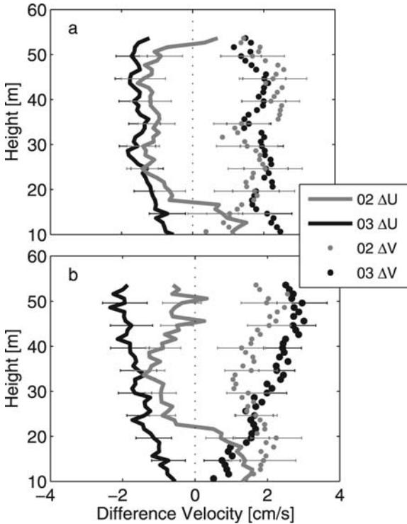
Figure 8. Profiles of alongshelf and offshore velocity differences during (a) descent and (b) ascent. Error bars indicate the standard deviation. Fitted velocities (Fourier method) were subtracted from measured velocities.
