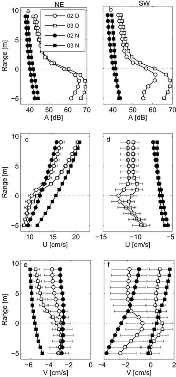
Figure 10. Profiles of amplitude, alongshelf, and cross-shelf velocity profiles and averaged background profiles half a lunar period away for northeast flow(a,c,e) and southwest flow (b,d,f). The upper boundary of the scattering layer is at a range of 0. Errorbars indicate twice the standard error.
