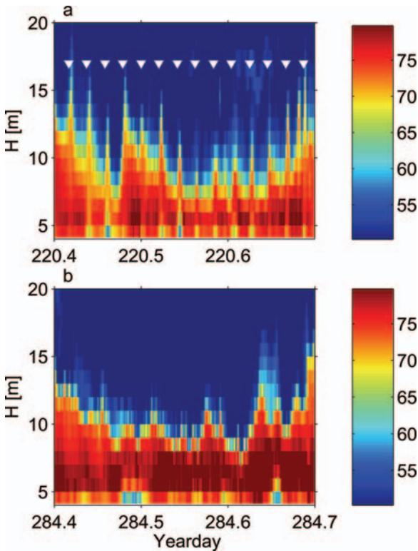
Figure 12. Backscatter amplitude for 2003, year days 220 and 284. White symbols indicate times when the light was briefly turned on.
