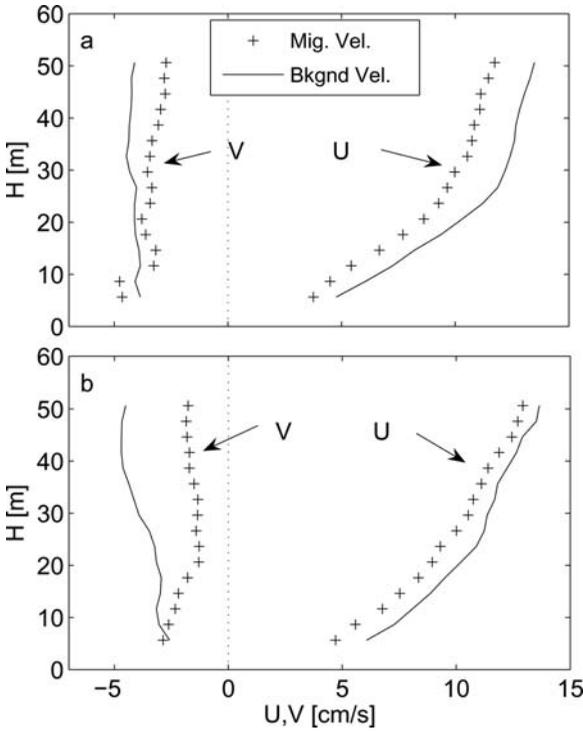
Figure 7. Profiles of experiment-averaged alongshelf and cross-shelf velocities during (a) descent and (b) ascent for 2003. Ambient velocity profiles are also shown.
